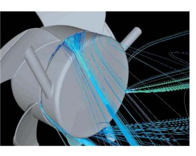
Calculation of airflow within the motor. Computer simulation is used to visualise the cooling air flow for sensitive operating points.
