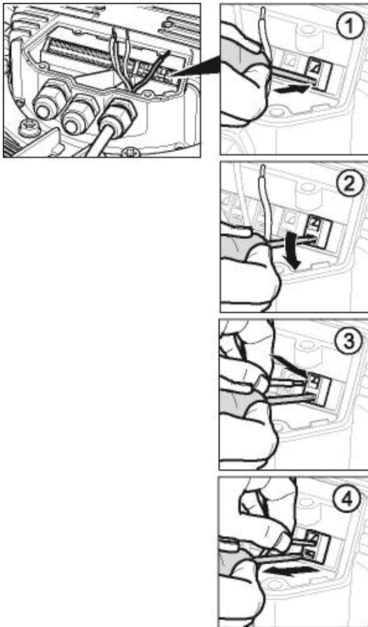
Fig. 2: Connecting the wires to terminals
